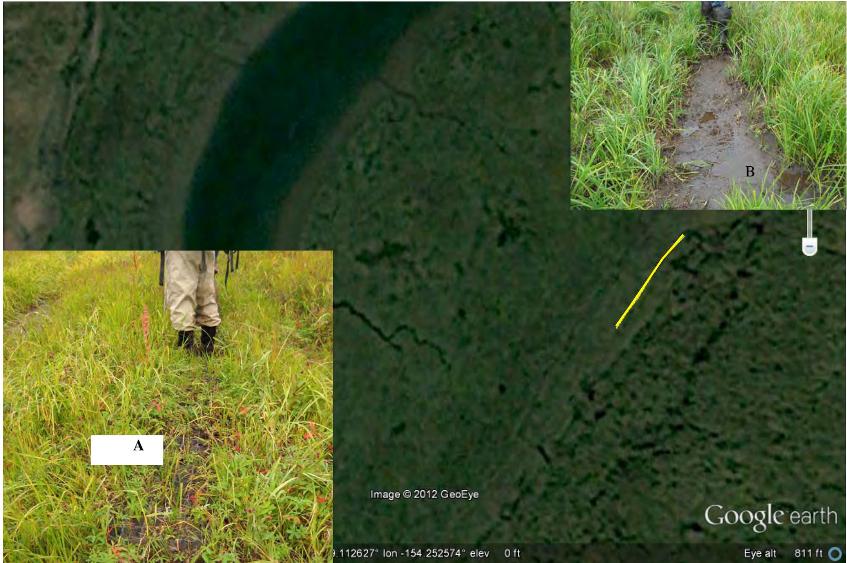
Figure 9. 2012 Geoblock trail stabilization, Mikfik Creek east side sedge meadows. Insets of treated (A) and untreated (B) trail sections.
